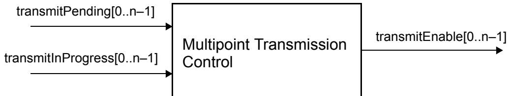
Figure 77-6—Multipoint Transmission Control service interfaces
