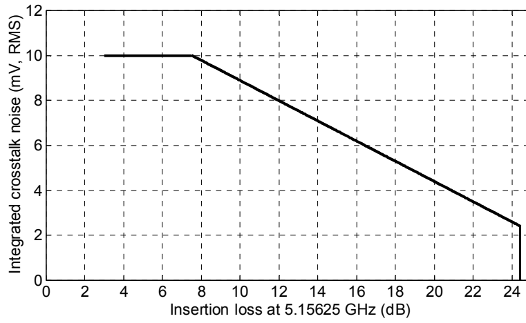
Figure 85A-2—Channel integrated crosstalk noise
